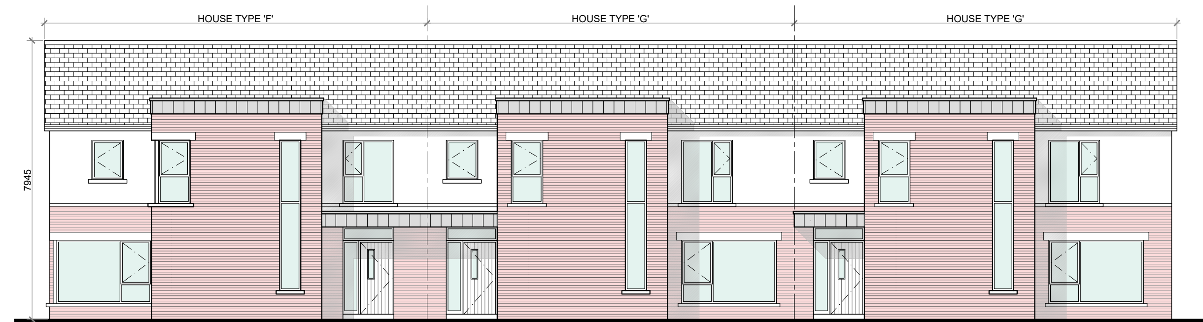
FRONT ELEVATION @ 1:100 TERRACE BLOCK TYPE 14
